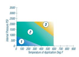
In area 1 the gasket material is suitable using common installation practices subject to chemical compatibility.
